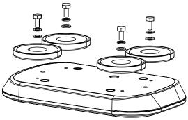
Four magnets are fixed with 4 screws at the bottom of the lightbar
