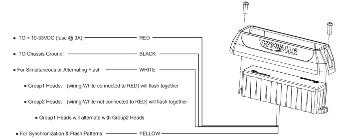
• Connect YELLOW wires of all heads together for synchronization
