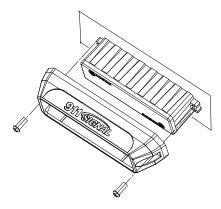
③ Install the LED module on the mounting surface by 2 screws
