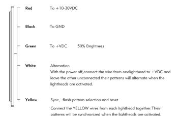
Flash patterns will be reset when YELLOW wires are connected to  $\pm$ VBAT for more than 5 seconds.
