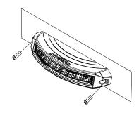
③ Install the LED module on the mounting surface by 2 screws
