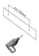
② Drill 2 holes on the mounting surface "
